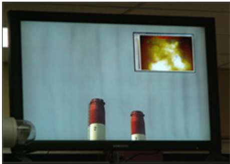
The combined ThermaScope and Video view in the control room. Engineers wanted to view smoke coming from the towers simultaneously with the thermal imagery
